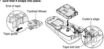
Make sure that the end of the tape feeds under the tape guides. • If the ink ribbon is loose, use your finger to wind the toothed wheel in the direction of the arrow on the cassette.
