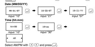
You can also confirm the figure and move to the next setting by using the right cursor key
