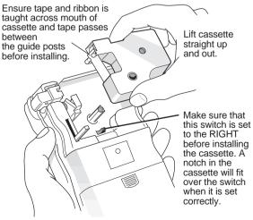
Push firmly until cassette clicks into place. Print head Label TAPE cutter -CASSETTE press to cut off (•) printed İabel.
