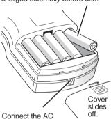
adaptor plug here. Use only the recommended adaptor. Plugging in the AC adaptor disconnects the batteries. Note: Re-chargeable batteries will not be charged.
