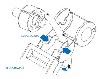
5 Insert the free end of the label roll, label side down, into the slot on the back of the printer. Push the label stock into the slot until you feel a slight resistance. Continue pushing gently. The SLP automatically feeds the labels through and aligns the end in the exit slot.
